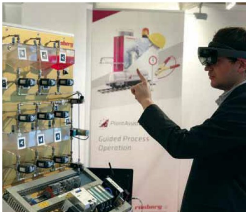
Figure 3: Graduate student Stefan Stegmüller uses a tank filling system to investigate the practical use of the Microsoft HoloLens for process industries.
