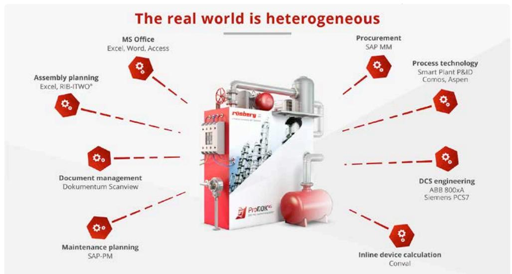
Figure 2: Revision-proof interfaces: Adapters convert data delivered by the other software tools involved in plant engineering, and pass them on to ProDOK NG.
